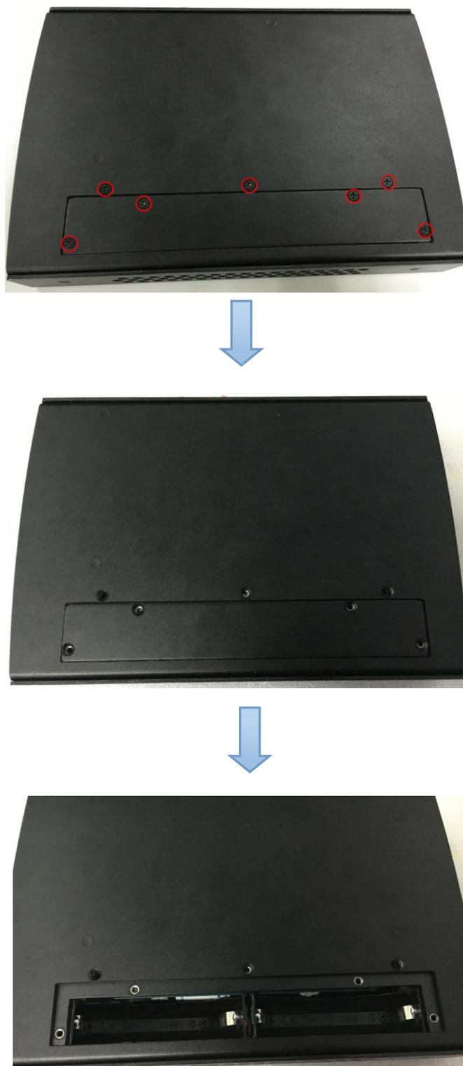
2. Prepare 2 lithium ion batteries. Pay attention to the positive and negative terminals of the batteries, this is the main points in installing the batteries. As shown in the figure below:
